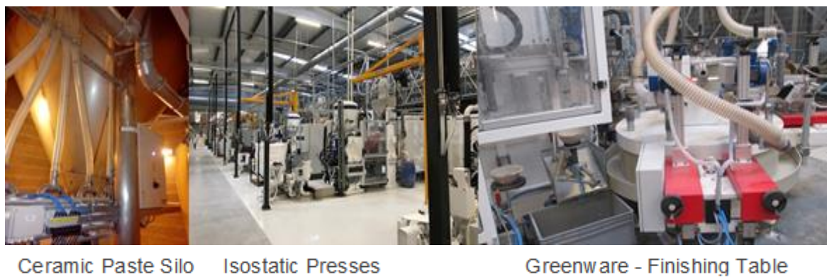
Figure 20. First stage of the production process: Silos, Presses and Finishing
