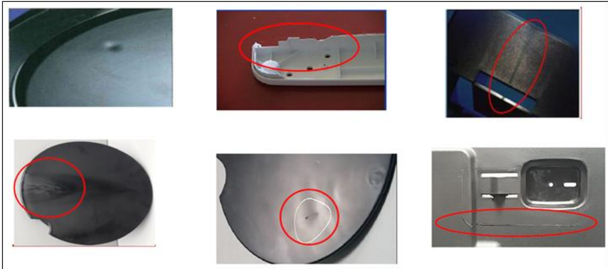
Figure 25. Injection visual defects a-Sink mark,b-short-shot,c-weld line,d-flow line-e-surface delamination,f-flash
